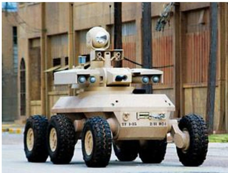
Figure 4. Lockheed Martin's Multifunctional Utility/Logistics and Equipment (MULE)<sup>34</sup>
