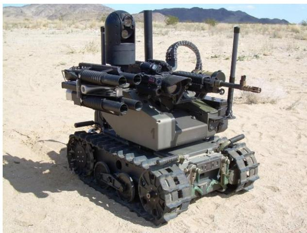
Figure 5. Qinetiq's Modular Advanced Armed Robotic System (MAARS)<sup>37</sup>
